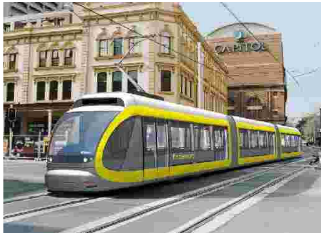
“Incentro” is the name for Adtranz' latest 100% low floor light rail vehicle designed specifically for operation in urban streets. Incentro will go into service on the Nantes, France urban light rail system, one of dozens of new systems built or under construction in Europe. Car floor is 11.2 inches above the rail.
