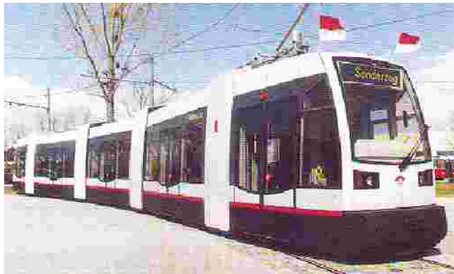
Modern low-floor trolley in Historic Vienna. In modernizing its extensive tramway system, Vienna selected the Elin ULF 197 ultra low floor tram. The trolley floor is only 7.8 inches above the rail, barely the lowest in operation anywhere in the world, making trams easy to board for travel in this historic European city.
