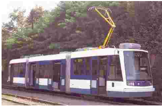
Low floor transit vehicles developed specifically for urban routes will soon be rolling on Portland Streetcar system. Shorter and lighter than high-speed LRVs used on most new U.S. systems, including Hudson-Bergen Light Rail now running in Jersey City and Bayonne, these cars would be ideal for crosstown operation proposed by VCTC. (Photo courtesy Skada)
