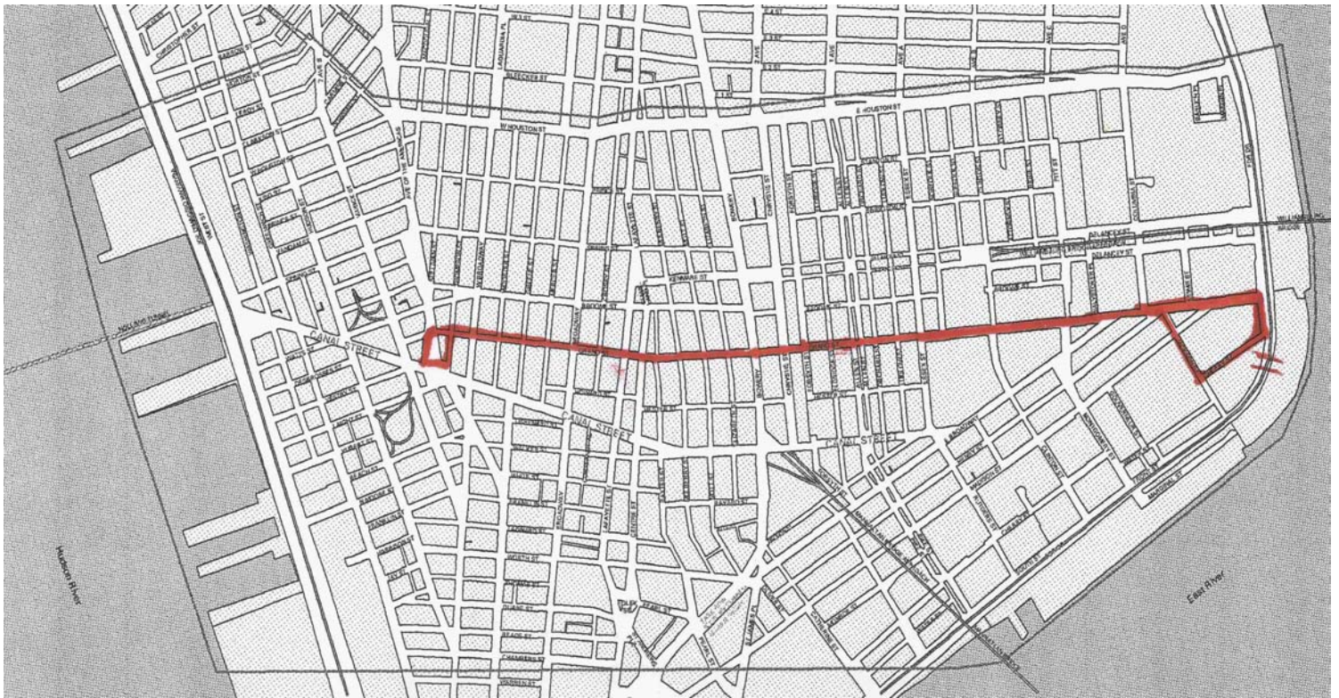
CATS map showing Grand Street light rail line. Western segment parallels Canal Street, providing haven for pedestrians and transfers to all major subway lines for riders from transit-starved lower east side. More than half of route lies east of Grand Street F line station, site of future 2nd Avenue subway connection should that 75-year-old dream ever be realized. Loops at ends of route provide direct access to subway stations and to East River Park, and will permit greater operating efficiency.
